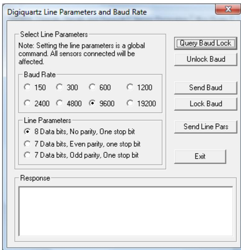
Each of the commands sent, by clicking a button on this dialog, is a global command that will be processed by all the sensors. The result from each sensor will be displayed. The baud rate lock must be off prior to changing the baud rate. During testing the line parameters of a sensor could not be changed. The response to a baud rate change is at the original baud rate. If the baud rate is changed, the driver's COM port baud rate must be changed before any other commands are sent.
