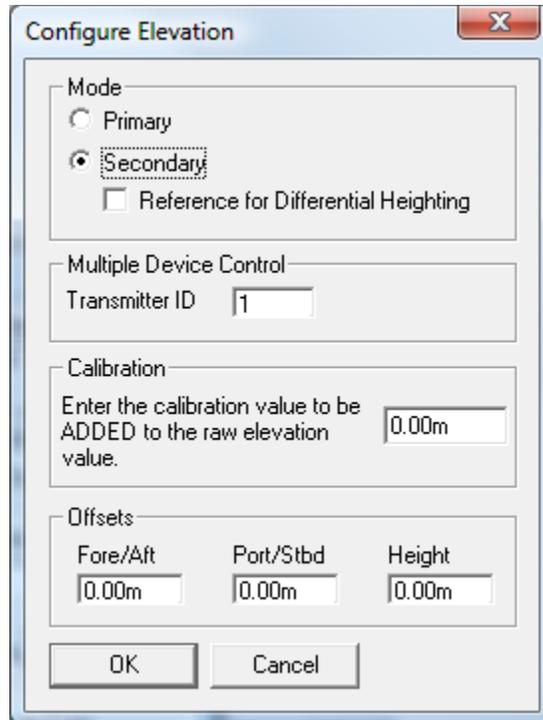
Set the mode to primary if this device is to determine the vehicles depth. The default is secondary. Other devices that can also determine depth need to be set to secondary for depth.
